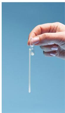
4. Add the milk into the pipette by squeezing the smaller upper bulb once, hold it, dip the pipette tip about 1 cm into the milk sample. Then release pressure on the bulb and the pipette (stem) will fill itself with the appropriate volume (0.25 ml) of milk. Note: After pipetting, the little surplus of milk is caught into the pipette reservoir (the small lower bulb). Repeat the pipetting when there is no milk in the reservoir or there are air bubbles in the stem.
