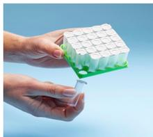
2. Detach one or more ampoules. Take care that the aluminum foil from the remaining tests is not damaged. Perforate the ampoules carefully.
