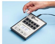
6. Check the temperature of the incubator (64°C +/- 2°C) and the set incubation time (7 minutes). Put the ampoules into the incubator.
