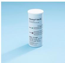
1. Take the strip container out of refrigeration (4-8°C recommended storage conditions) and allow the container to warm up to room temperature.
