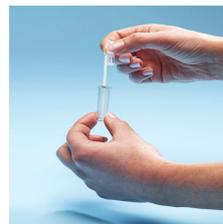
5. Transfer the milk sample by gently and totally squeezing the same upper bulb, adding the milk straight in the ampoule. Note: The little surplus of milk in the lower bulb will remain. Shake for +/- 30 secs. until all reagents are dissolved.
