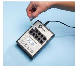
7. Take one test strip; immediately close the container containing the strips. Hold the test strip from the upper side (green area). Insert one test strip per ampoule. Once inserted start the incubator timer.
